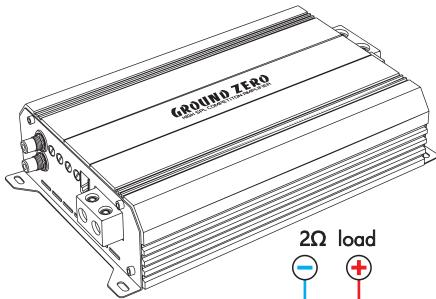
Serial wiring @ 2Ω load
