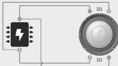
Parallel / serial mixed wiring → 2 Ohms
